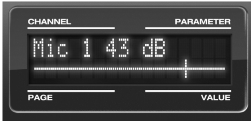
Figure 4-5: The LCD gives you feedback as you turn the TRIM knobs for the two mic/guitar inputs.
