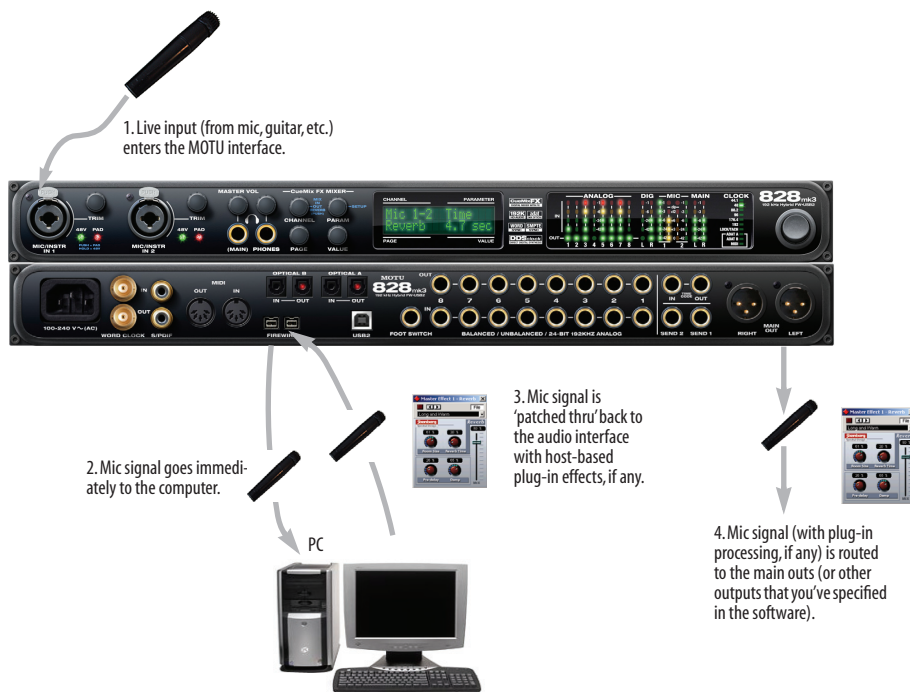
Figure 8-1: There are two ways to monitor live audio inputs with an 828mk3: 1) through the computer or 2) via CueMix FX hardware monitoring. This diagram shows method 1 (through the computer). When using this method, use your host software's buffer setting to reduce the slight delay you hear when monitoring the live input, but don't lower it too much, or your computer might get sluggish.
