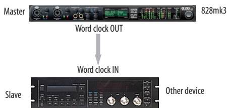
Figure 4-19: Slaving another digital audio device to the 828mk3 via word clock. For the 828mk3 clock source, choose any source besides word clock, as it is not advisable to chain word clock.
