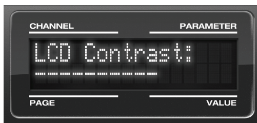
Figure 6-5: In setup mode, the LCD displays a setup parameter in the top row of the LCD and the current setting in the bottom row.
