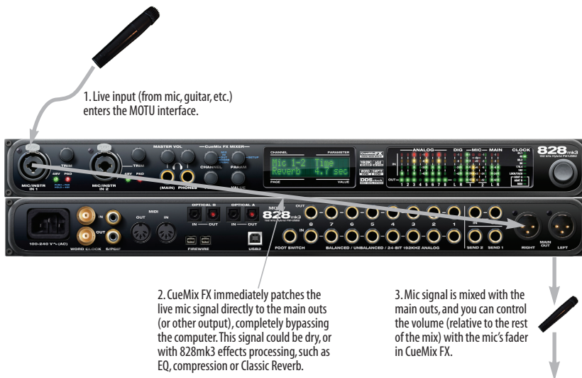
Figure 8-2: This diagram shows the signal flow when using CueMix FX no-latency monitoring. Notice that this method does not process the live input with plug-ins in your audio software. Instead, you can apply 828mk3 effects, such as the reverb, EQ and/or compression.
