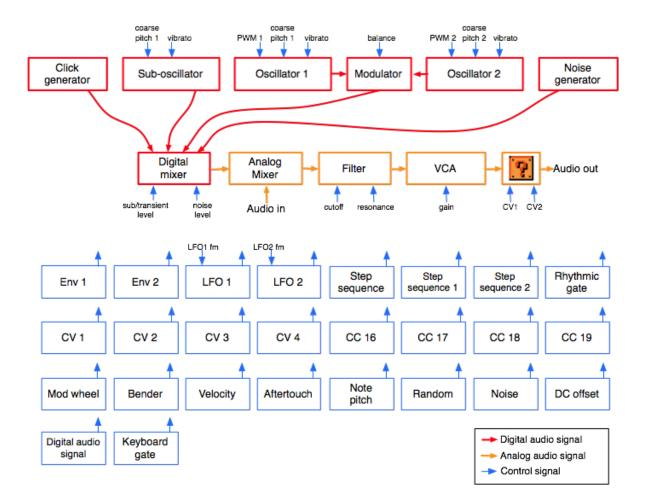
The audio signal flow is represented in red (digital path) and then in orange (analog path):
