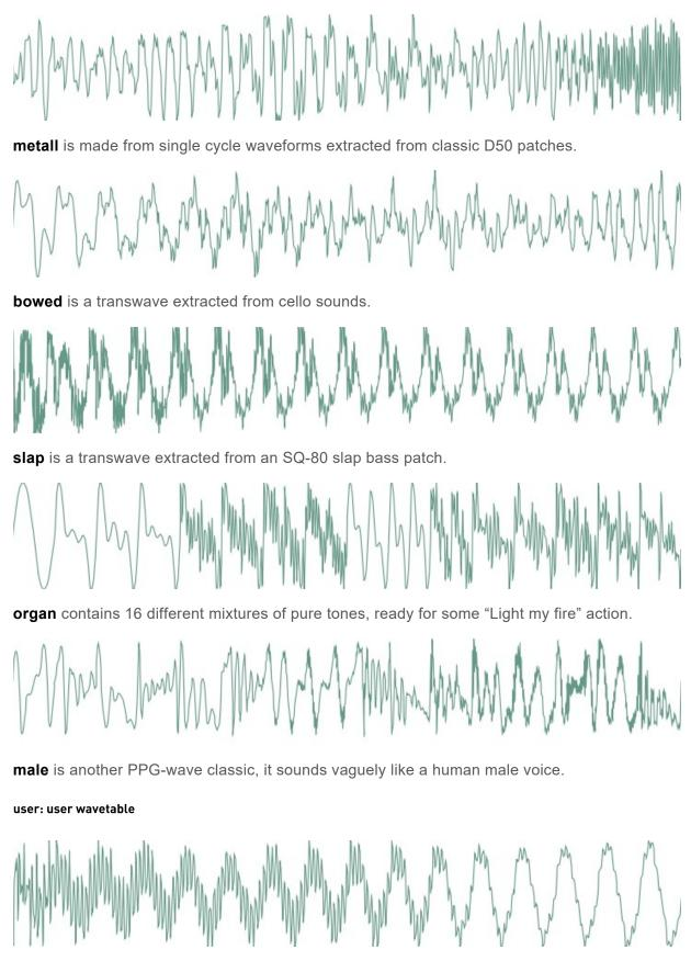
This wavetable has two peculiarities: it is smaller than the other ones (8 single cycle waveforms, each of them being 129 samples long), and it resides in RAM instead of residing in flash ROM. By default, it is loaded with the same content as **digitl**, but its content can be altered by <u>SysEx messages</u>. You can find <u>here</u> some examples of MIDI files containing user wavetables.
