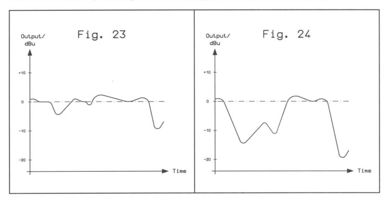
Compressor 1 (fig. 23) and compressor 2 (fig. 24) AFTER gain control
