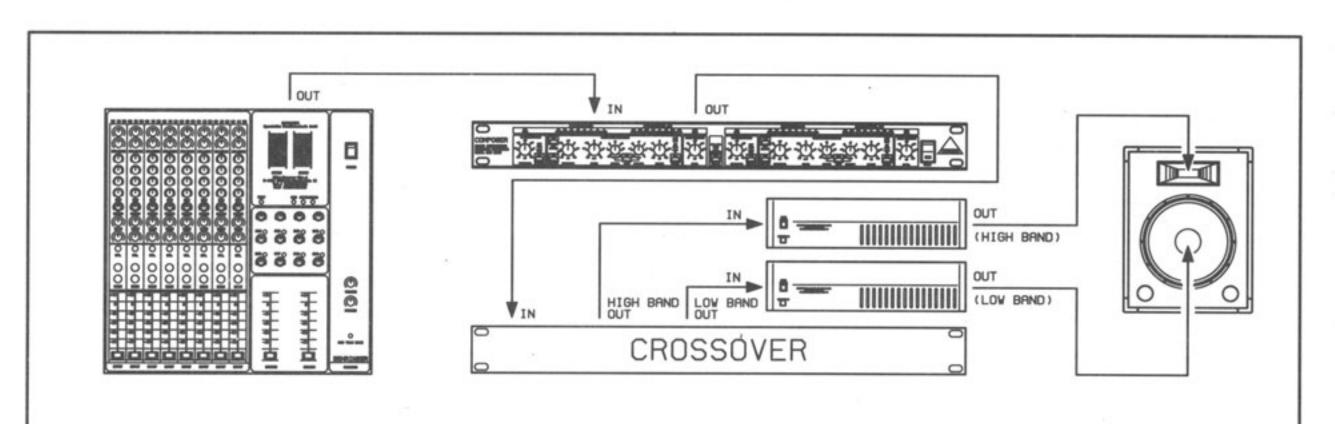
Fig. 31 The Behringer COMPOSER in a two way system
