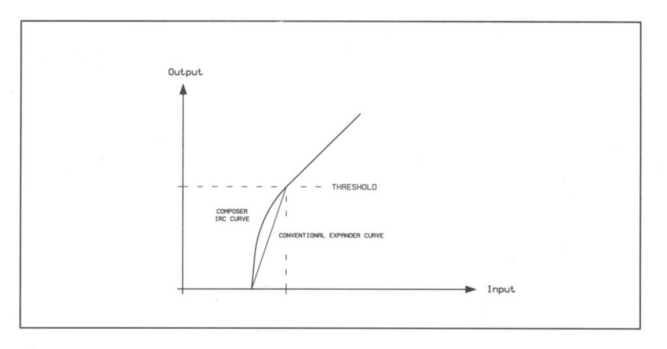
Fig. 17 IRC curve characteristics of the Expander
