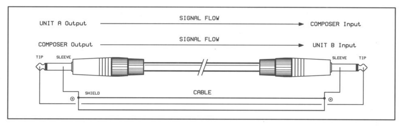
Fig. 10 Unbalanced input and output wiring with 1/4" jack connections
