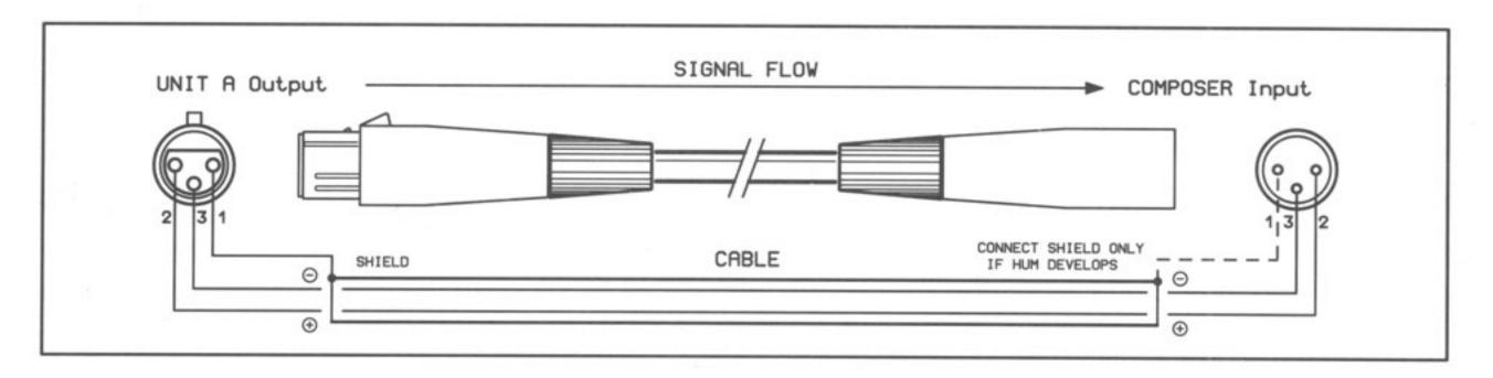
Fig. 5 Balanced COMPOSER input wiring using XLR connectors
