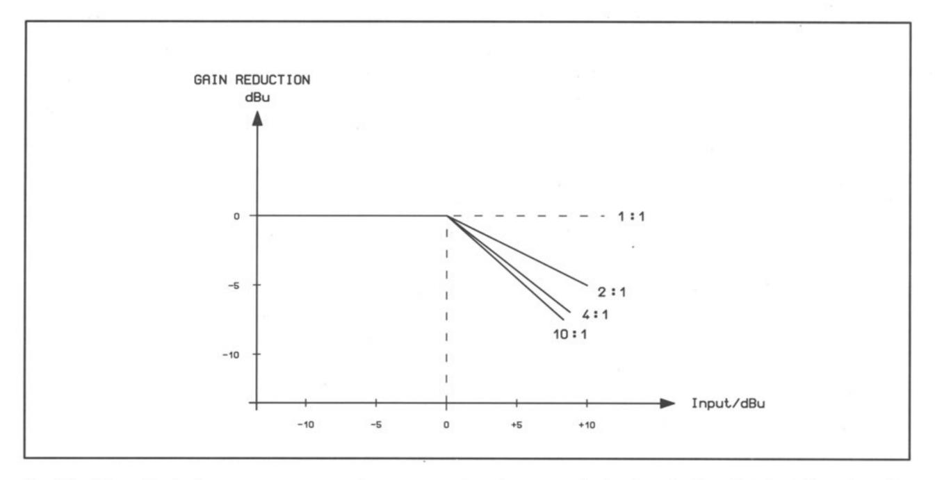
Fig. 20 The effect of a compressor can be expressed as the amount of gain reduction that is taking place for any given input
