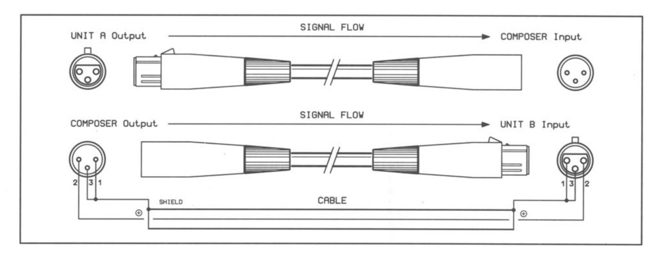
Fig. 7 Unbalanced input and output wiring using XLR connectors
