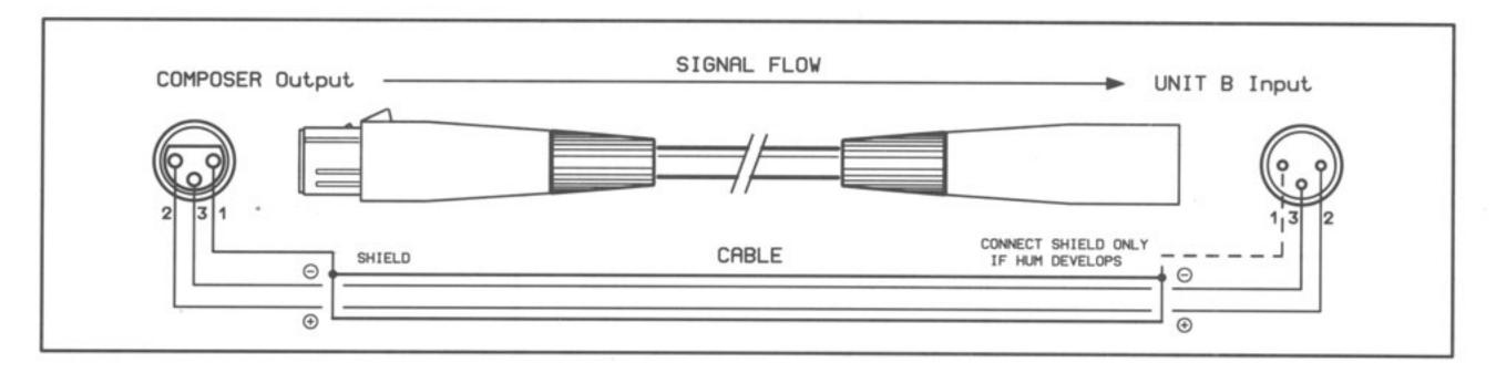
Fig. 6 Balanced COMPOSER output wiring using XLR connectors
