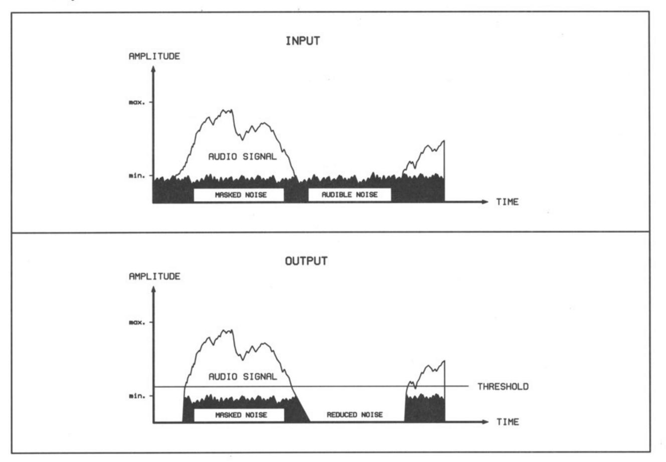
Fig. 16 Function of an expander
