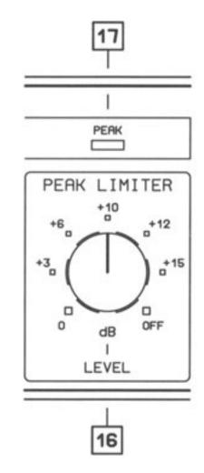
Fig. 14 Control surface of the Peak Limiter section
