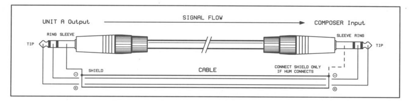
Fig. 8 Balanced COMPOSER input wiring with 1/4" jack connections
