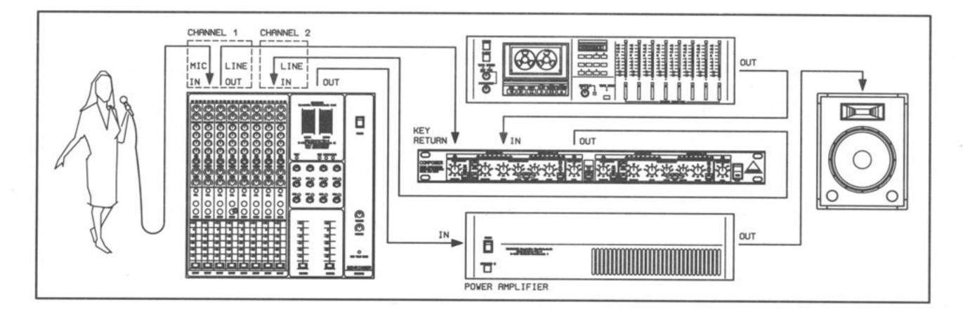
Fig. 37 "Voice-over" compression using the Behringer COMPOSER
