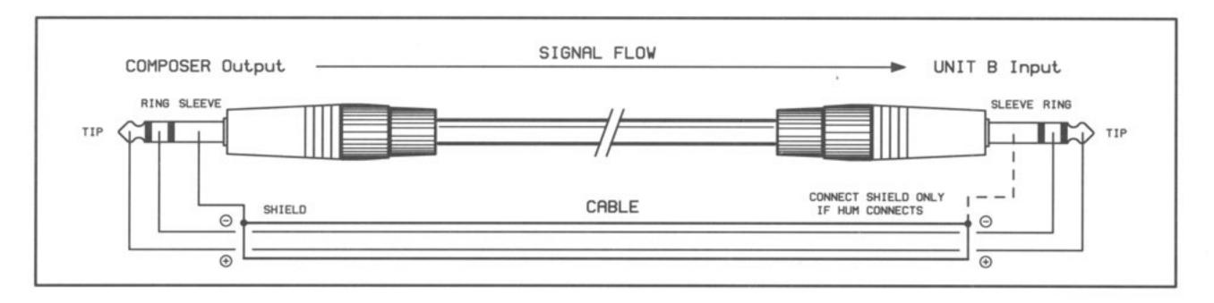
Fig. 9 Balanced COMPOSER output wiring with 1/4" jack connections
