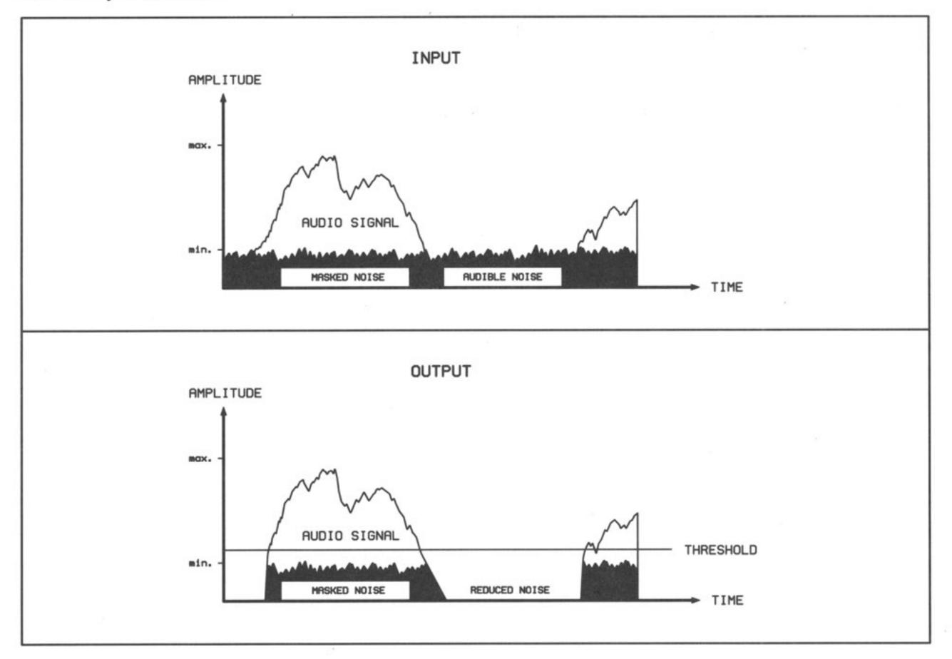
Fig. 16 Function of an expander
