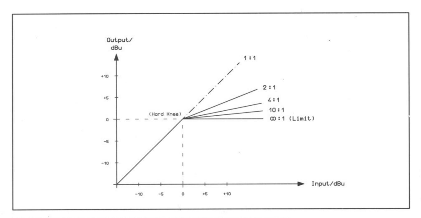
Fig. 18 The ratio of input to output level with reference to different ratio settings
