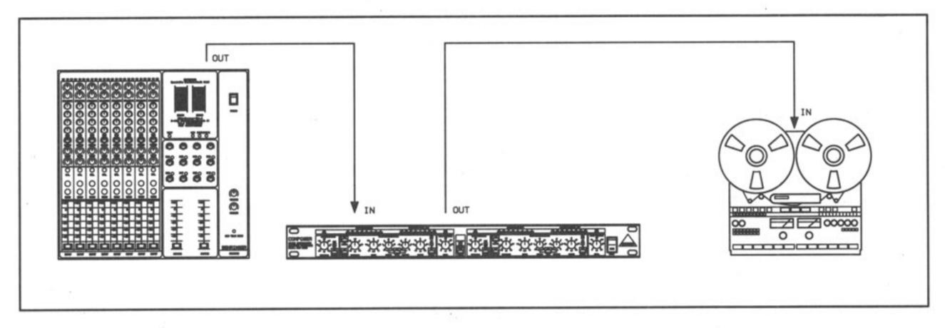
Fig. 33 Using the Behringer COMPOSER to avoid distortion due to tape saturation
