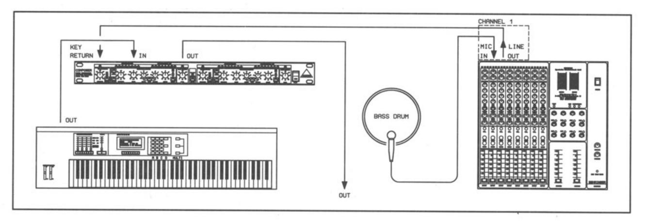
Fig. 38 Triggering a keyboard sound using a bass drum
