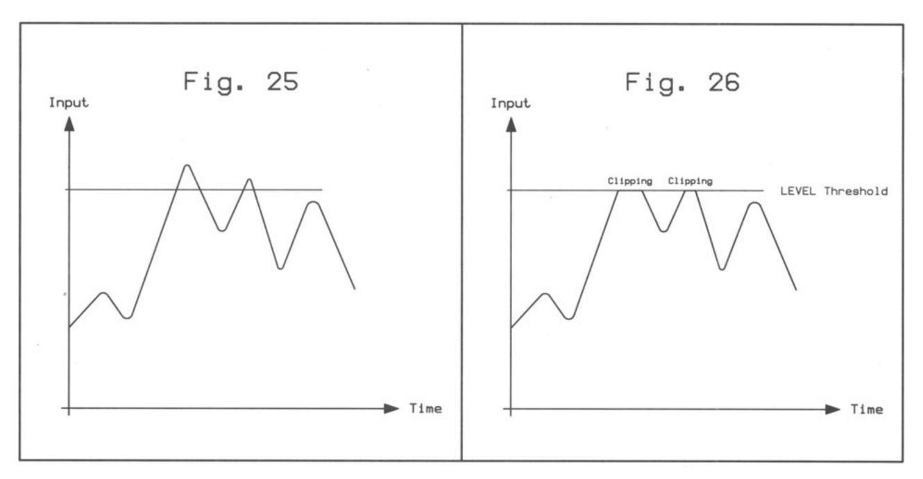
The signal BEFORE gain control (fig. 25) and AFTER clipper processing (fig. 26)
