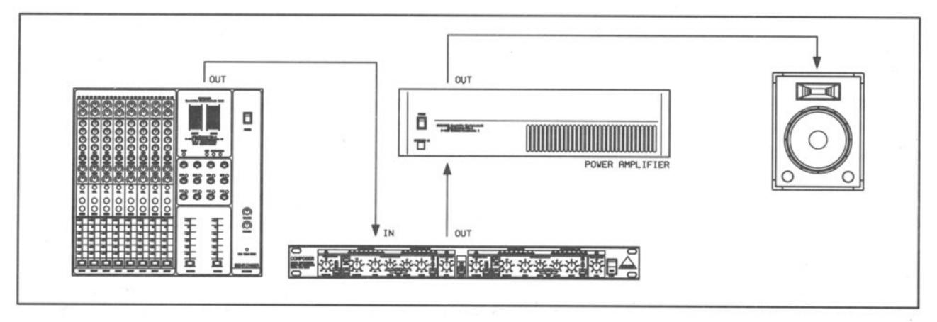
Fig. 30 Integrating the Behringer COMPOSER into a system with a passive crossover network
