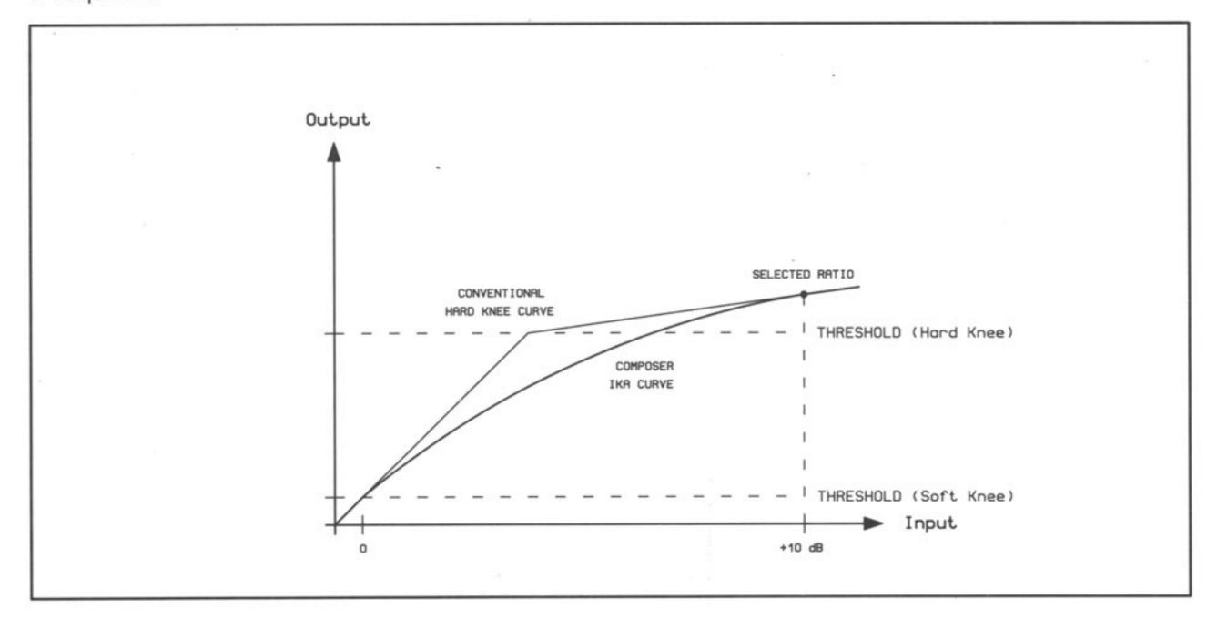
Fig. 19 Curve characteristics of the IKA circuit
