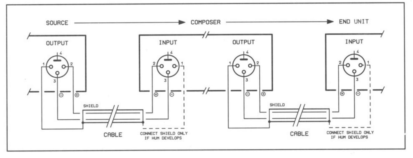
We recommend that you connect the shield of the input cable with the ground of the signal source, making sure that the shield is *not* connected to the COMPOSER's input connector.
