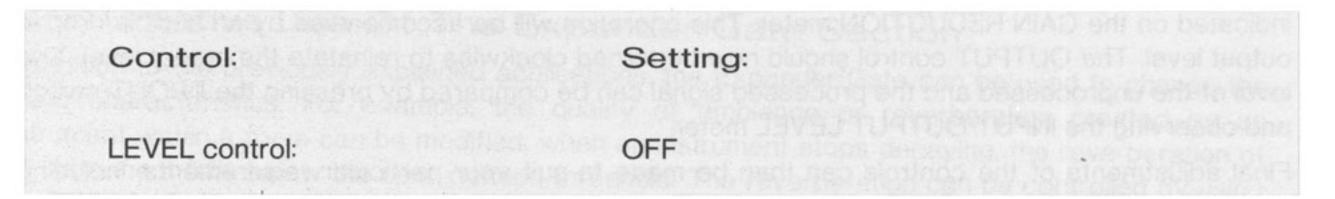
The LEVEL control of the Peak Limiter sets the threshold level, so that subsequent units are protected from overloading. If the PEAK LED comes on regularly or is on constantly, the OUTPUT control of the Compressor section must be turned down, as this control sets the level of the signal, which is routed to the Peak Limiter section.
