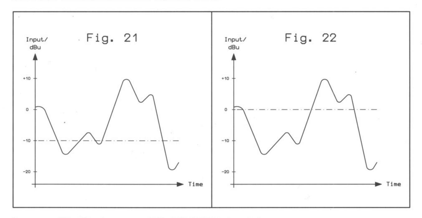
Compressor 1 (fig. 21) and compressor 2 (fig. 22) BEFORE gain control
