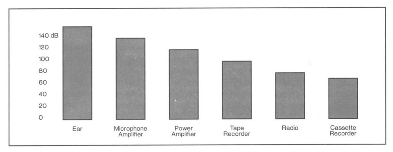
Fig. 1 The dynamic range capabilities of various devices
