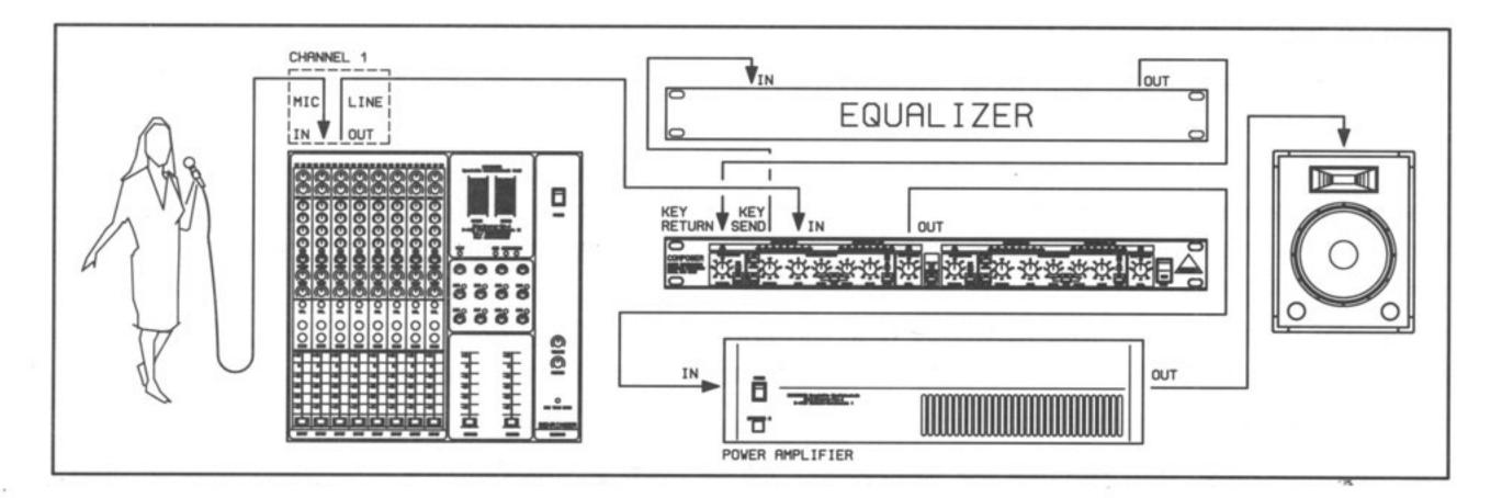
Fig. 34 "De-essing" using the Behringer COMPOSER
