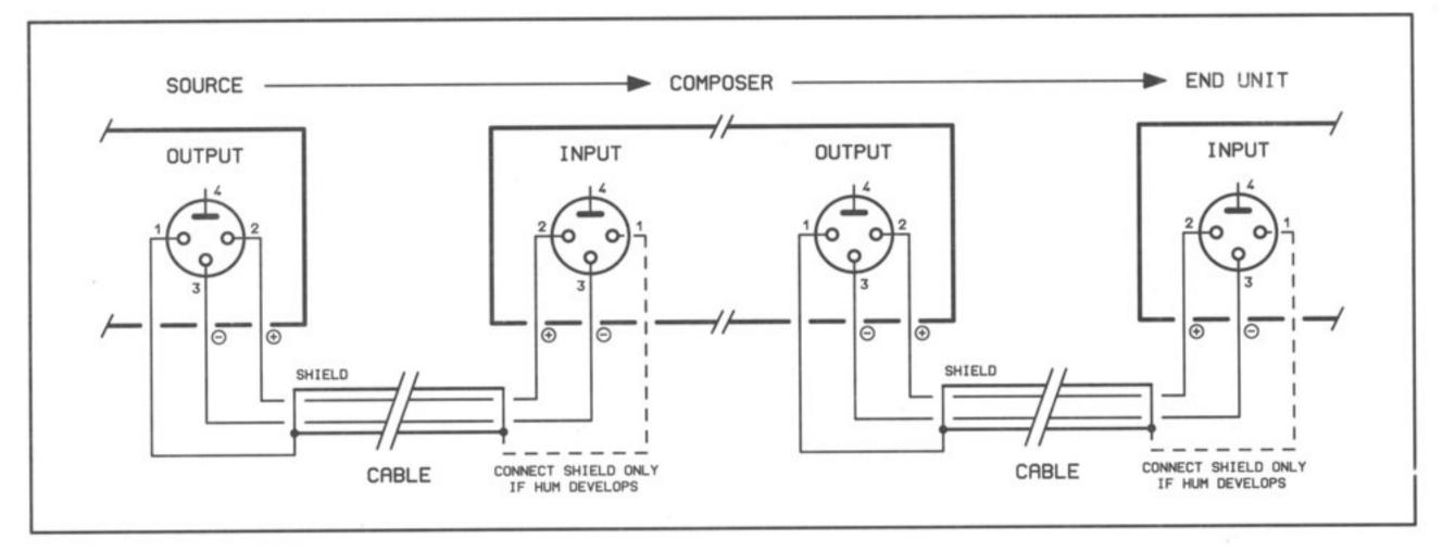
Fig. 4 The correct wiring of the balanced system
