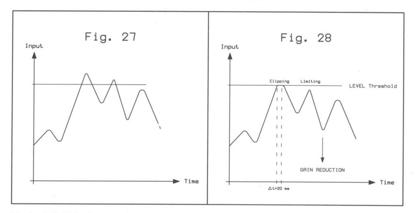
The signal BEFORE gain control (fig. 27) and AFTER IGC peak limiting (fig. 28)
