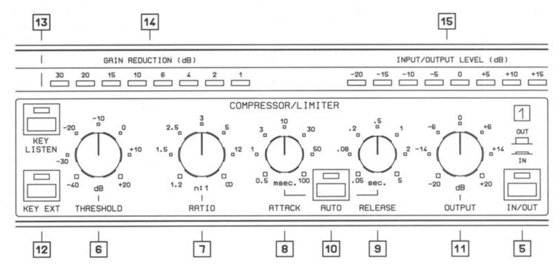
Fig. 13 Control surface of the Compressor section
