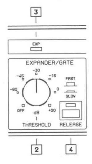
Fig. 12 Control surface of the Expander/Gate section
